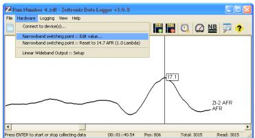
Open the Zeitronix Logging Software. Connect the Zt-3 Wideband AFR Meter into a PC COM port or USB to serial adapter and power up the Zt-3. Make sure the log graphs are shown on the screen. Open the Narrowband Switching Point menu by selecting Settings/Narrowband Switching Point.
