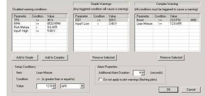
lower than 3.4V. Also, a warning will be activated if the AFR mixture will be leaner than 12.8 AFR **AND** at the same time the boost level exceeds 23 PSI. The alarm is kept for additional 4 seconds to cool the engine down.
